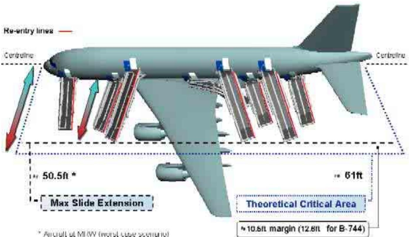
vertical holds and at tip for night evacuation, as well as "re-entry" lines for access of ARFF crews to both decks in case of absence of other means (illustrated below). The slides extend 50.5ft from the longitudinal centerline of the fuselage, which is only 3.2ft more than B747 upper deck slides. The clearance obtained between the far end toe of upper deck slides and the TCA perimeter is 10.5ft (aircraft at Maximum Ramp Weight).
