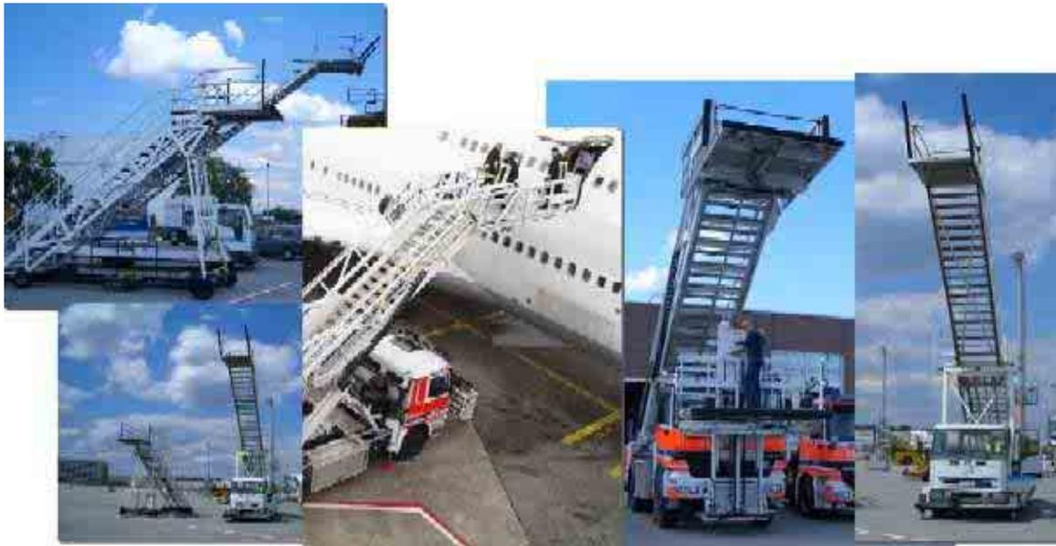
ARFF upper deck access vehicles used by Frankfurt ARFF for B747 operations, while other portable stairs capable of reaching 8m height (same as B747 upper deck doors) are also illustrated.
